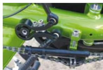
two fingers, they don't squash any fingers you've left wrapped around the bars. Challenge say the shape of the CNC-machined lever has been somewhat refined for extra comfort since ours were made, though I didn't have any complaints. Each brake is fitted with a spring-loaded 'parking' lock.
